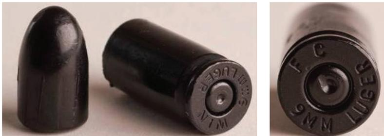
The resin bullet and cartridge case castings are now ready for ballistic imaging or comparison microscope examination and comparison.
