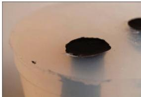
Place the resin-filled mould into the pressure pot and close the lid. Connect the air compressor to the pressure pot. Turn on the air compressor and apply 30 psi of air pressure to the pressure pot. Allow for the resin to cure for about 2 hours in the pressurised pressure pot. Check the exact time required by the resin manufacturer.
