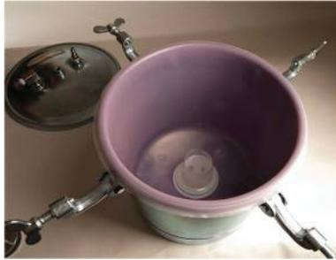
Close the pressure pot and connect it to the air compressor. Turn on the air compressor and apply 30 psi of air pressure to the pressure pot.
