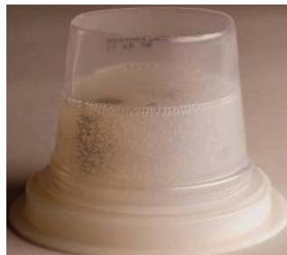
Place the mould box into the pressure pot.
