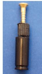
**Take care not to damage the mould and the bullet/cartridge case.** The base portions of the cured resin bullet and cartridge case castings can be removed with a small razor saw or can be cut off on a small lathe taking care not to damage the cured resin bullet and cartridge case castings.
