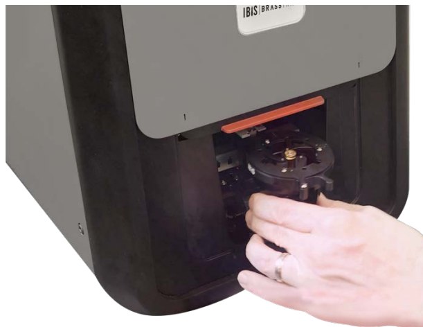
Figure A6-9 – IBIS BRASSTRAX Acquisition Unit (Inserting a Cartridge Case Holder)
