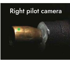
Within the Left and Right pilot camera views, the green dots indicate the acquisition camera's field of view. Set a target point using red crosses in the pilot camera views. Navigate to the target point using 'Move-To' button on toolbar.
