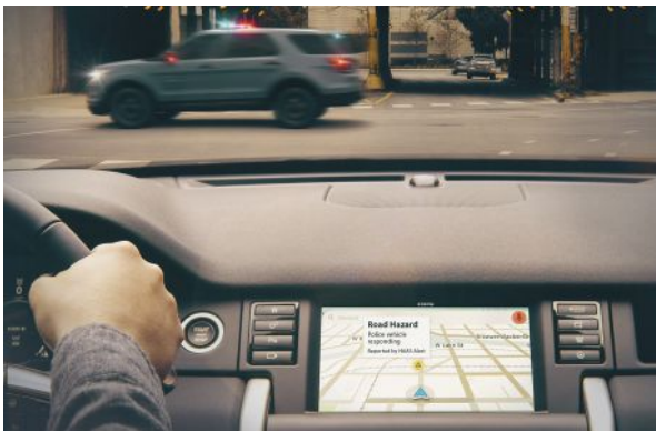
HAAS Alert's Safety Cloud lets motorists know that emergency vehicles are in operation nearby. The alert system can be activated by lightbars or other devices in the first responders' vehicles.
